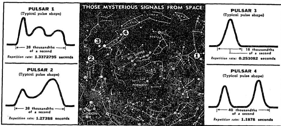
Observations with the radio telescope at Arecibo, P. R., have shown that three of the "beeping" objects recently discovered (map) have much in common. They are known as Pulsar 1, Pulsar 2 and Pulsar 4. All repeat their pulses at intervals of slightly more than one second and each pulse lasts from 38 to 40 thousandths of a second. Each also has its characteristic pulse shape (single, double or triple) when displayed on an oscilloscope. Pulsar 3 differs from the others. All may be neutron stars.
